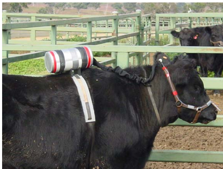
Figure 3. Steer fitted with methane collection apparatus. (From: Hegarty et al. 2007)
